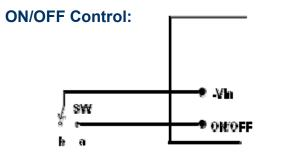
The converter output can be disabled by moving SW to position "a"– connected to –Vin with voltage level between -0.7 and 0.4V.
